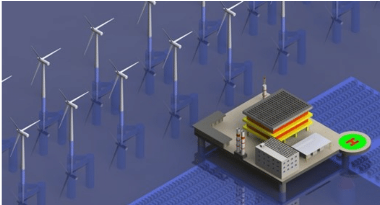
Figure 3-9 Platform Conceptual rendering of platform in combination with offshore wind energy devices and solar panels. Combined installations of wind and solar energy were currently only considered for the self-sustainability of the platform rather than for provision to land. Source: Tiong et al., 2015
